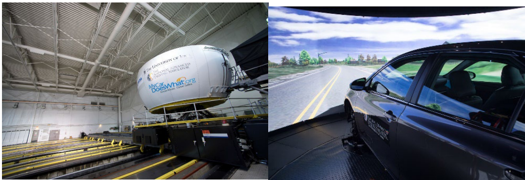
Figure 3.1 NADS-1 dome—exterior (left), interior (right)
