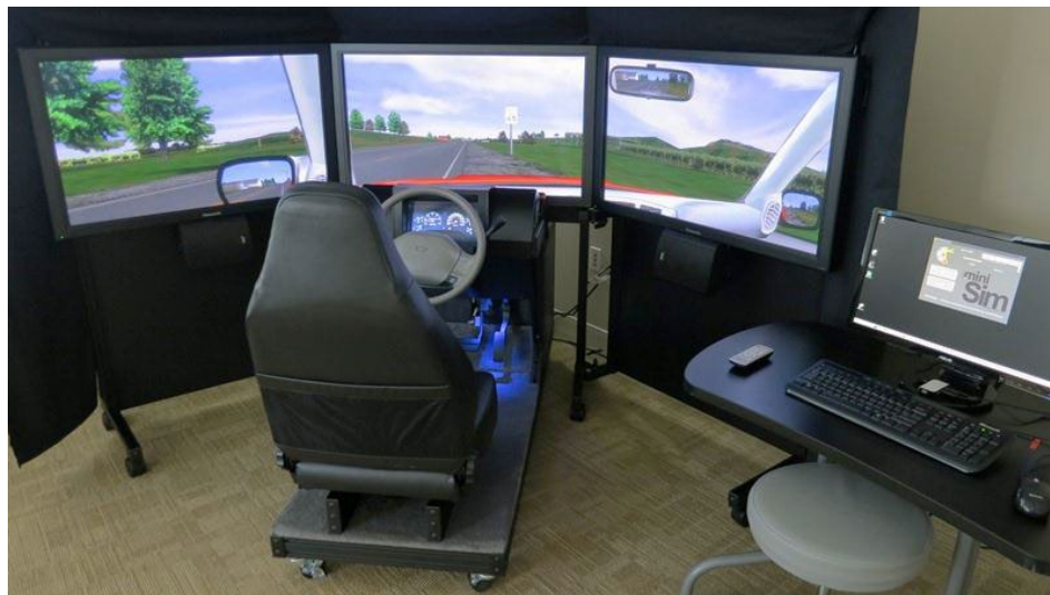
Figure 3.2 miniSim driving simulator with a quarter cab
